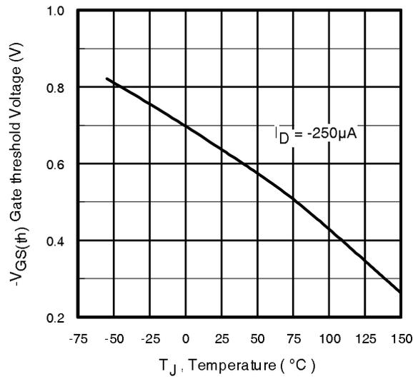
**Fig 15.** Typical V<sub>gs(th)</sub> Vs. Junction Temperature
